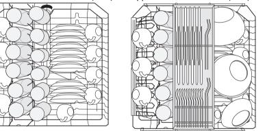
\* If necessary, move the cup rest from right to left. When doing this, ensure that the cup rest is at the same height.
